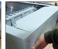
Lift up the paper pusher platform
