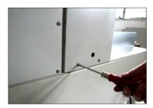
◆ Loose five M8 fasten screws on the blade carrier which fixed the blade and adjust the adjustable screw on blade carrier, until the blade cuts into the cutting stick about 0.3-0.5 mm;
