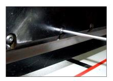
◆ Adjust the support chip on the screw, and you can move it back and forth until digital display dimension matches measuring scale dimension, then lock the retaining screw firmly.
