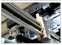
◆ Pull out the front covering strip, and check stepping motor, to see whether the synchronous pulley and synchronous belt are fixed normal;
