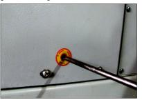
◆ If the last paper still can not be cut completely after fine adjustment the cutting blade depth. Adjust the balanced screw of cutting blade depth once more. Disassemble retaining screws on both sides of the upper cover, and then take the upper cover away;
