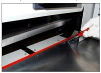
\* Note: When knife shim is being changed, the blade itself also needs to be adjusted. If the blade cuts too deep, the knife shim will be damaged easily. and also the blade will abrade rapidly.
