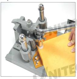
Place sheets and align them tightly to both sides of the side guides, push handle downward to cut.
