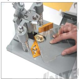
Calibrate and fix the side guides by using the alignment board.
